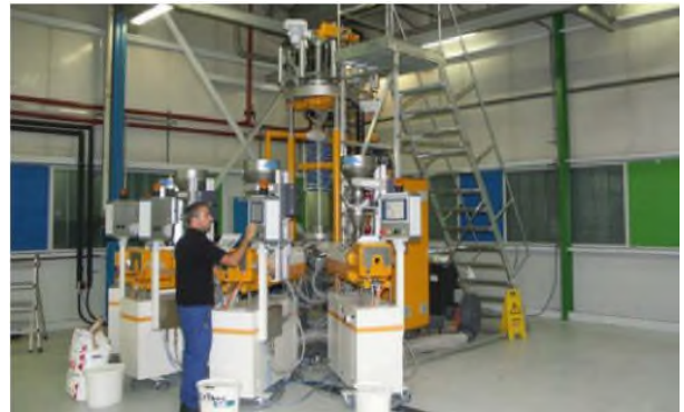
The computer-controlled pilot plant can produce high-quality film adhesives on a laboratory scale.
